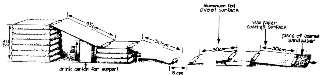
**Wheels and Axles** materials: pint-sized carton; meterstick; pushpins; stir straws; 4 platforms from push-up ice cream (wheels); posterboard (30 cm x 45 cm); masking tape; large straws; scissors; 6 hardcover books
